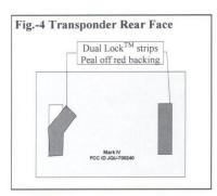
The transponder may be removed by lifting any one corner with sufficient pressure to separate the Dual  $Lock^{\mathsf{M}}$  strips. Do not remove the Dual  $Lock^{\mathsf{M}}$  from the windshield and reuse it; obtain new strips from your service center if necessary.
