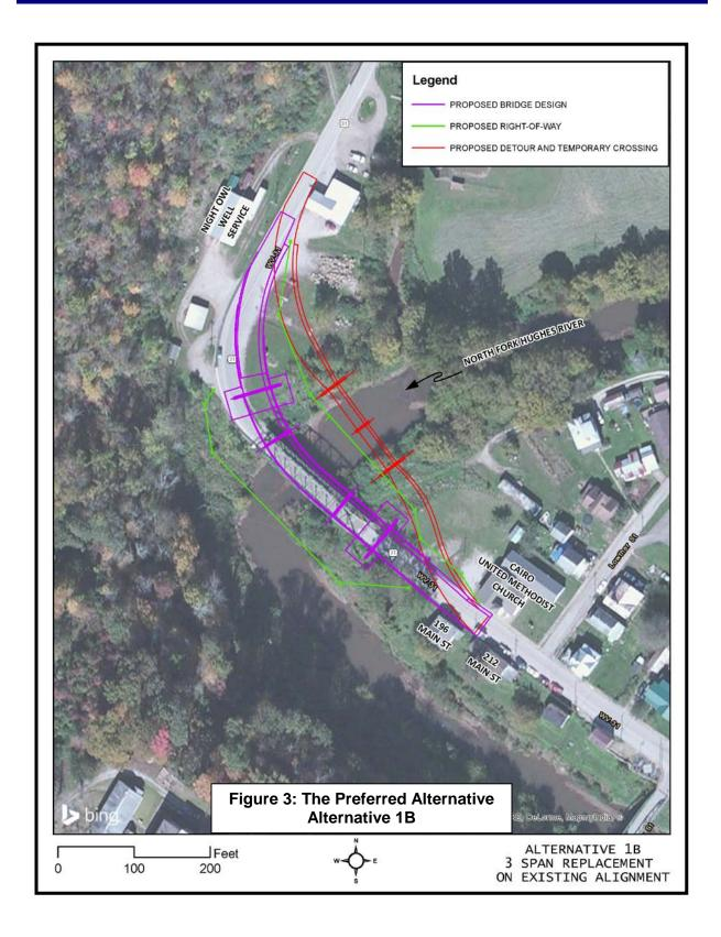
Alternative 1B will replace the existing Cairo Bridge on the same alignment currently used. The new bridge will have two 11-foot travel lanes and a 5-foot sidewalk. It will have three equidistant
