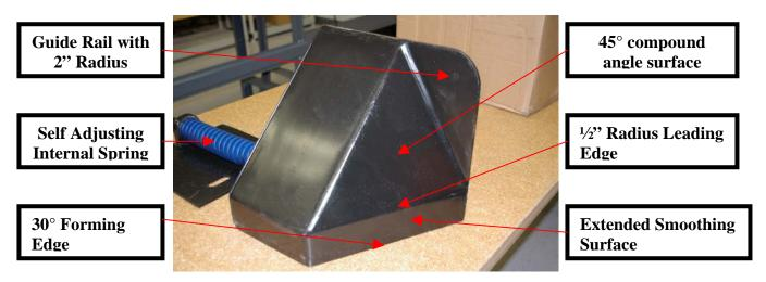
The Guide Rail allows the Shoulder Wedge Maker to ride along the surface of the road shoulder following its topography. The 2" radius helps the transition when the device encounters an obstacle such as a driveway cut or road intersection.
