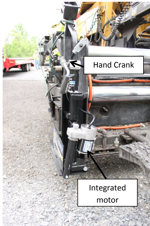
Figure 8: Hand crank and motor controlled angle adjustment
